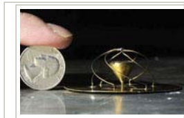
At a size comparable to a quarter, the ultra-wideband antenna is cheap and simple to produce, according to one of its inventors, Taeyoung Yang.
