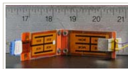
Energy harvesters are small devices that convert other forms of energy to electricity.
